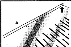
To secure the cover to the wall, drill two holes into the wall and attach with two screws.
